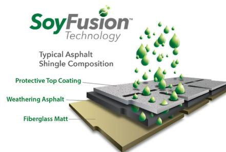
shingles, making them inflexible. SoyFusion Technology allows millions of microdroplets of oil to quickly penetrate the brittle protective top coating and saturate the weathering asphalt layer. This infusion rejuvenates the asphalt, restoring its flexibility and pliability. Roof Maxx also enhances adhesion of the protective mineral granules, which work like sunscreen, reflecting the sun's ultraviolet rays, the main source of physical/chemical degradation of roof materials.
