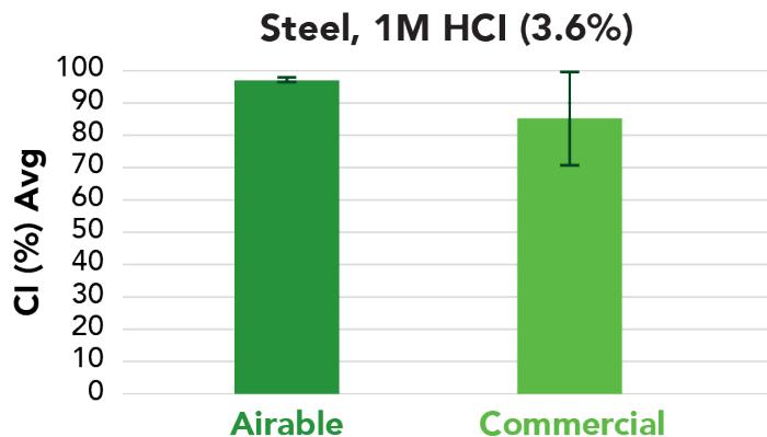
Steel coupons were submerged in 1M HCl solutions with and without inhibitor for 24 hours. The mass loss was used to calculate corrosion rate compared to the negative control.
